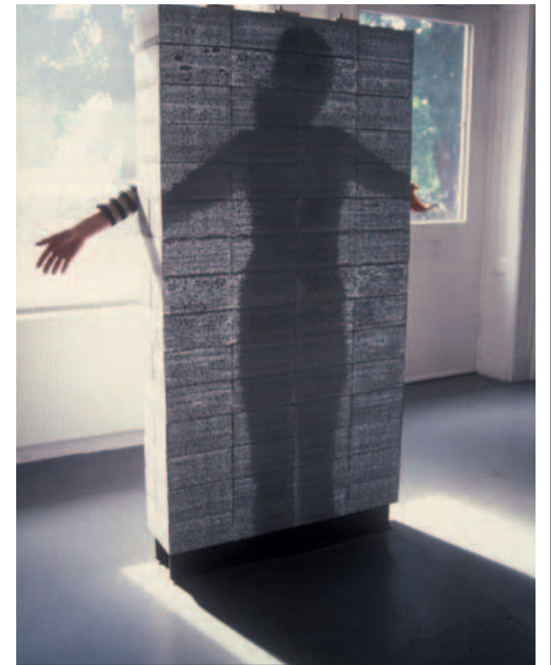
Looking through a concrete wall. Light-transmitting concrete blocks can be embedded with luminous optical glass fibres. At up to 500 mm thick, the blocks can be used to build a wall several metres in thickness. Light information from one side of the concrete, such as a shadow, is replicated by optical fibres embedded in the opposite side © Litracon
